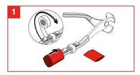
Slide Gripp Shrink over Tool Catch and V-Gripp Tape, ensuring that the D-ring is left exposed and accessible.
