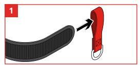
To connect to a work belt, thread work belt through the loop.
